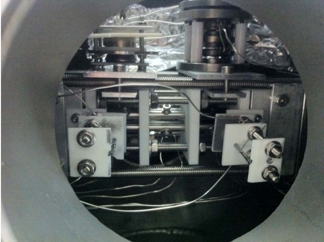
Figure 3. Ion trap in vacuum chamber
